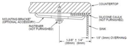
NOTE: THIS UNDERMOUNT SINK IS DESIGNED TO MOUNT TO SOLID SURFACE (NON-LAMINATE) COUNTERTOP ONLY.
